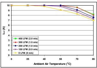
Figure 5: Maximum output power derating curves vs. ambient air temperature for airflow rates of 0 LFM through 400 LFM with air flowing across the converter from pin 3 to pin 1 (nominal input voltage).
