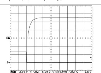
Figure 9: Turn-on transient at full load (resistive load) (10 ms/div). Input voltage pre-applied. Ch 1: Vout (2V/div) Ch 2: ON/OFF input (5V/div)
