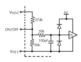
Figure B: Internal ON/OFF pin circuitry
