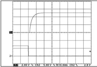
Figure 10: Turn-on transient at zero load (10 ms/div). Ch 1: Vout (2V/div)
