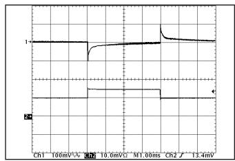
Figure 12: Output voltage response to step-change in load current (50%-75%-50% of Iout(max):  $dI/dt = 5A/\mu s$ ). Load cap: 470 $\mu F$ , 30 m $\Omega$  ESR tantalum capacitor and 1µF ceramic cap. Ch 1: Vout (100mV/div), Ch 2: Iout (5A/div).
